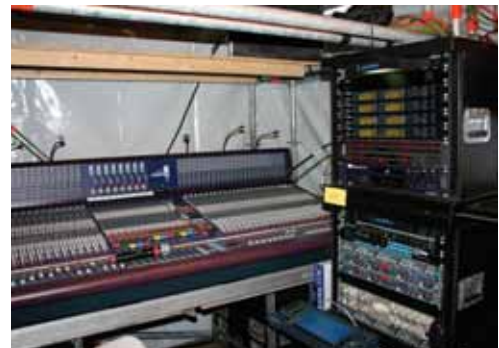
Above, a row of Robe 1200 Wash units. Marengi notes, "Much of the equipment was installed in technical troughs, sitting approximately 1.5m [4.92] off the ground, working on the theory that the closer the light was to artists, the fewer problems there would be with fog obscuring beams." Below: The monitor mixing position, with the Midas Heritage 4000 console
